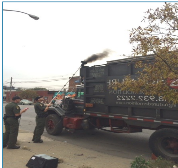
NYSDEC Environmental Conservation Officers measuring opacity of diesel emissions.
