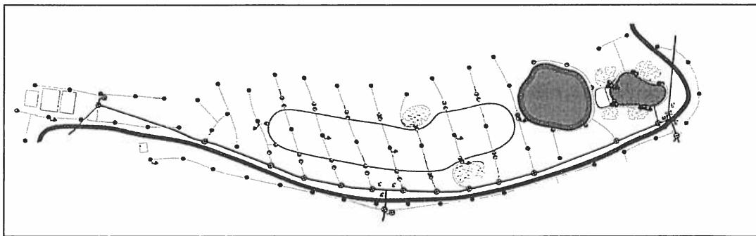
*Figure 1: Sample modern irrigation layout giving golf course superintendent ability to water the fairways and rough separately. Notice how the irrigation more closely follows line of play.*
