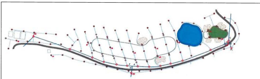
Figure 10: Sample modern irrigation layout giving golf course superintendent ability to water the fairways and rough separately. Notice how the irrigation more closely follows line of play.
