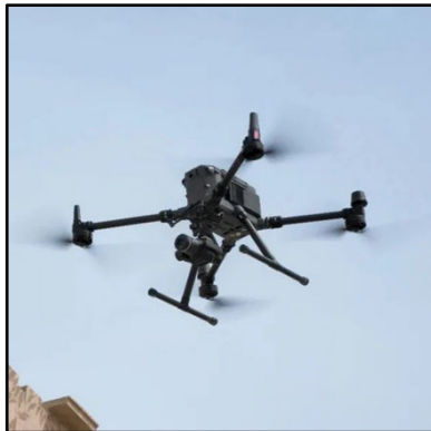
Figure 1: The DJI Matrice w/ Photogrammetry Sensor
